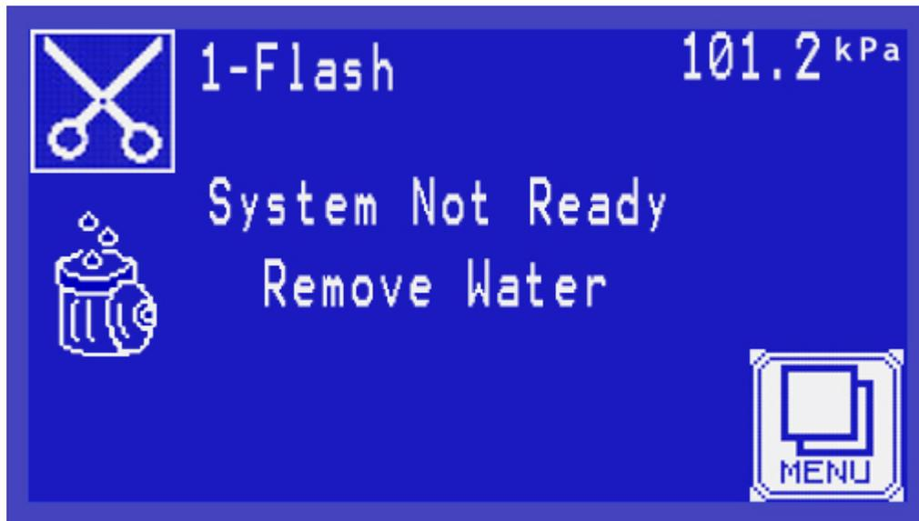
If the machine is not ready to perform sterilization process, the reason will be displayed on Stand-by screen. In this case, the 'START' key is unavailable. If the device is ready to perform sterilization cycle, "Ready" message is displayed and 'START' key is visible.
