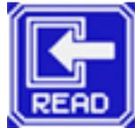
Pressing the 'READ' key will replace current selected field value with value of the analog input.
