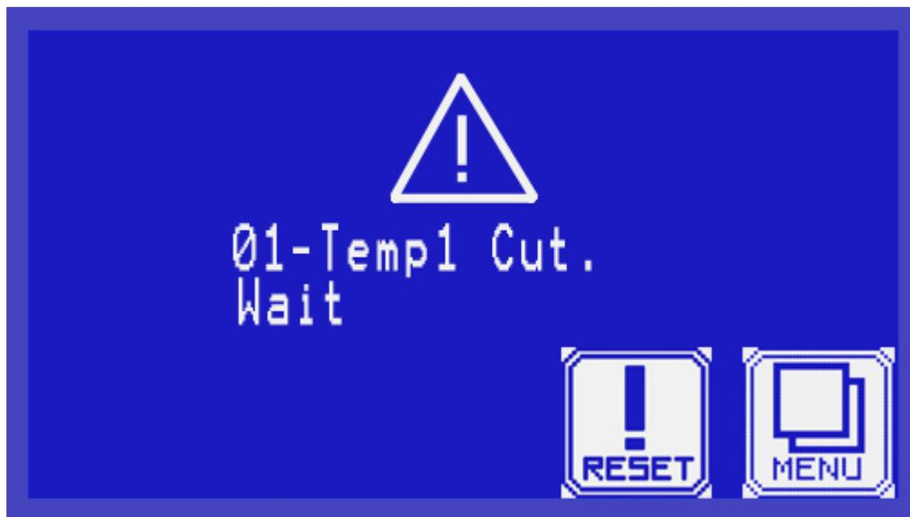
If an error occurs, or a sterilization process fails, the reason will be displayed. The system will not respond until the 'RESET' key will be pressed.
