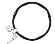
Press the remaining sections of the seal.
