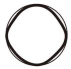
Press in the left and right sides of the door seal.
