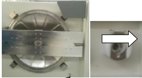
Water tank outlet a
